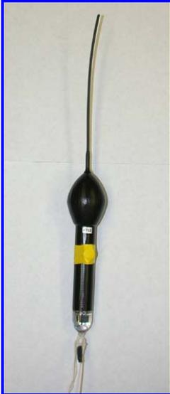
The satellite pop-off tag weighs about two ounces, and features a main body that is just over 13 inches in length and 0.8 to 1.6 inches in diameter. It carries an eight-inch nylon coated stainless steel antenna.
